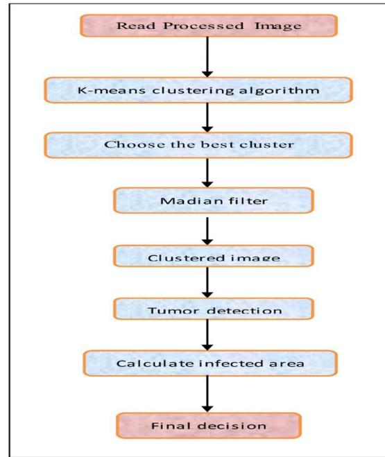
Figure 2. Block diagram of proposed k-means algorithm.
