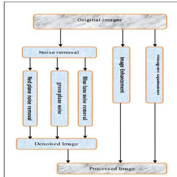
Figure 1. Block diagram of pre-processing stage.
